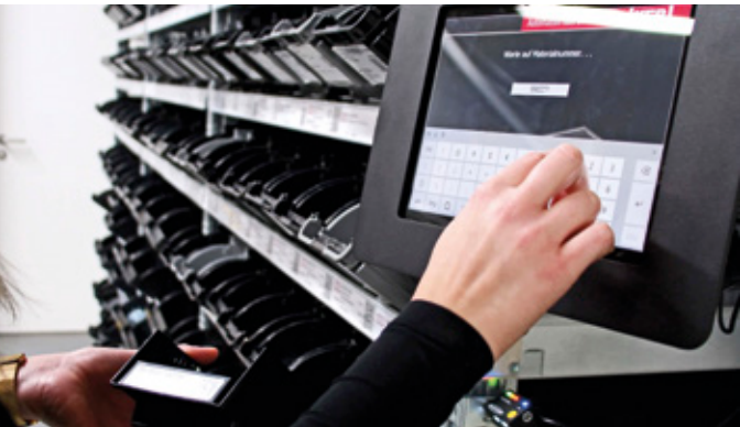
The KEB controller developed in-house, runs on a Windows tablet attached to the shelf
