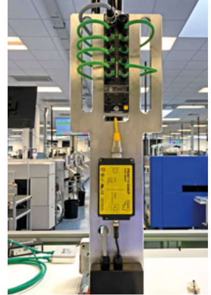
Robust and compact: The IP67 power supply unit and the IP67 switch provide a cabinet-free connection between the sensors and the MES
