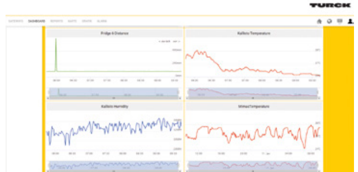
Predictive maintenance: The observation of temperature and humidity over long periods of time allows conclusions to be drawn about the wear of seals
