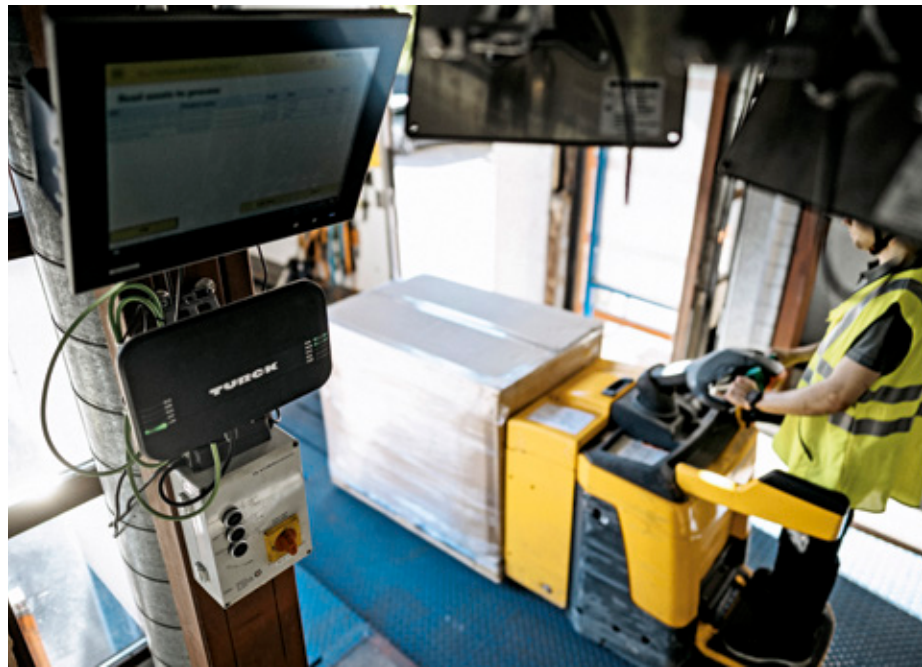
The RFID readers are designed to read multiple RFID tags simultaneously, for example, a pallet of RTIs moves through a gate
