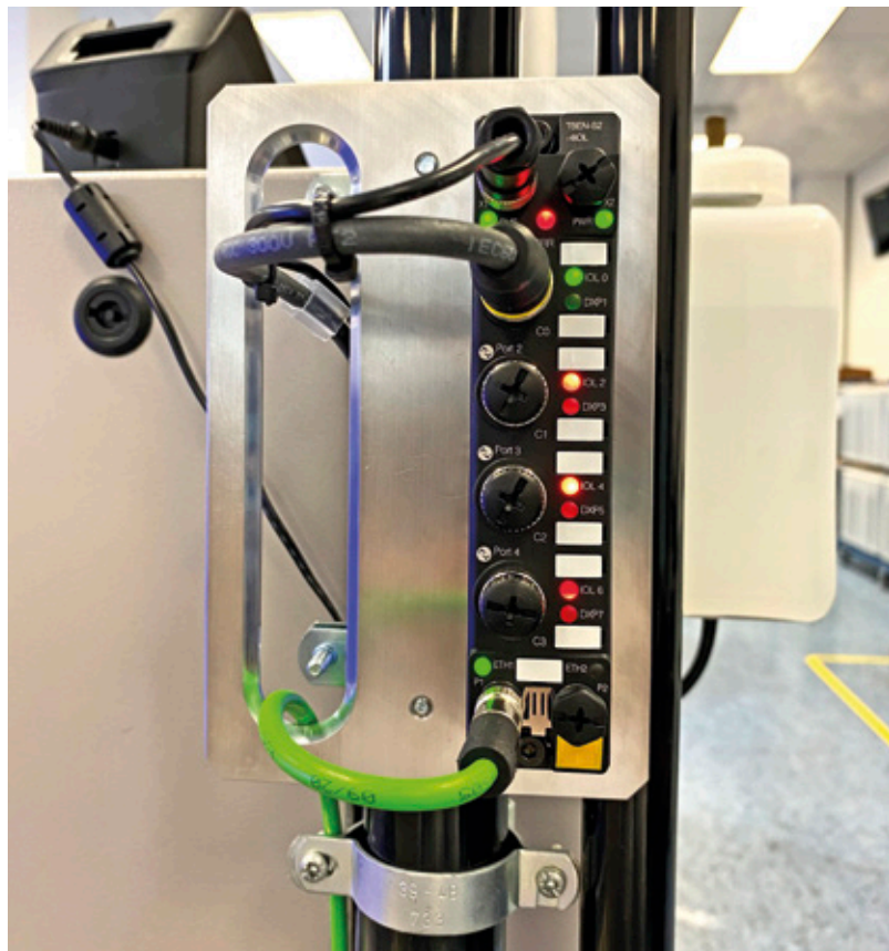
“Brain” of the system: The Linux-based IM18-CCM (CCM stands for Cabinet Condition Monitoring) bridges the gap between OT and IT
