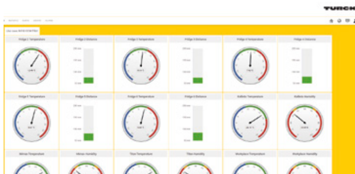
The graphical dashboard makes it possible to see the status of the refrigerators and the other workstations at a glance
