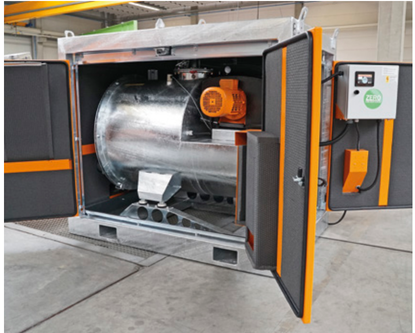
The water from the soil is temporarily stored in the tank and from there pumped into a body of water or the sewerage system
