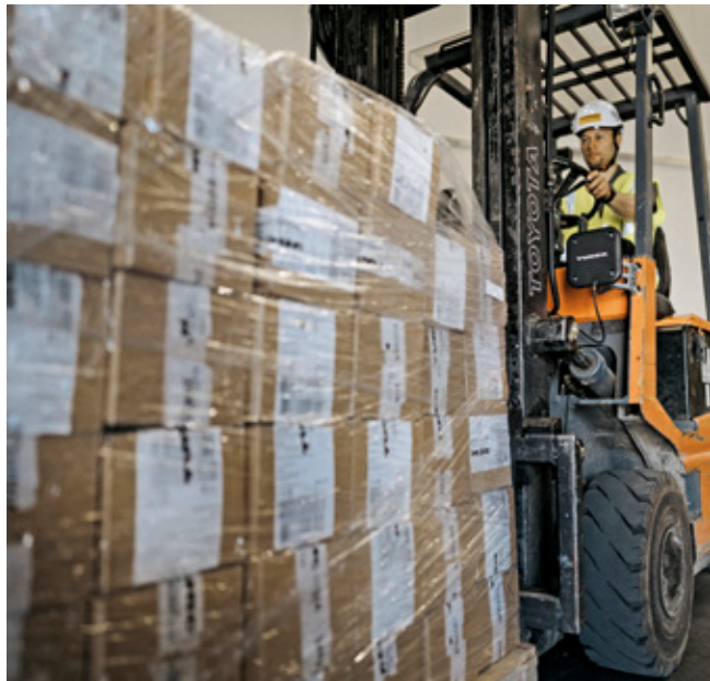
The forklifts equipped with RFID readers allow reliable and fast identification of pallets and containers
