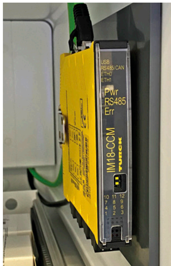
“Brain” of the system: The Linux-based IM18-CCM (CCM stands for Cabinet Condition Monitoring) bridges the gap between OT and IT
