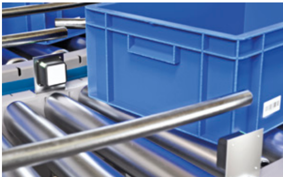
Barcodes are a relatively inexpensive identification technology, but they are more difficult to automate – especially if several containers are to be read simultaneously
