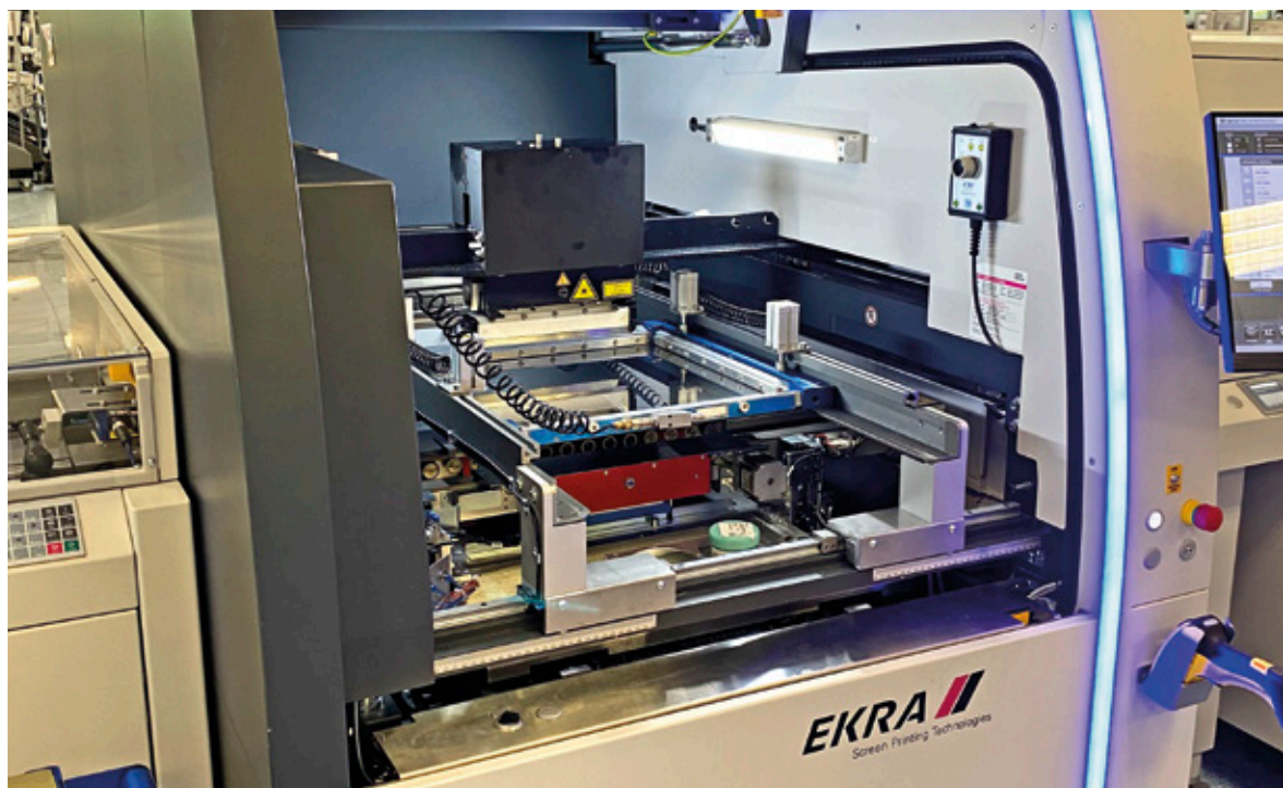
The solder pastes are inserted in the front area of the printer, and the CMTH sensor directly next to it detects the ambient conditions
