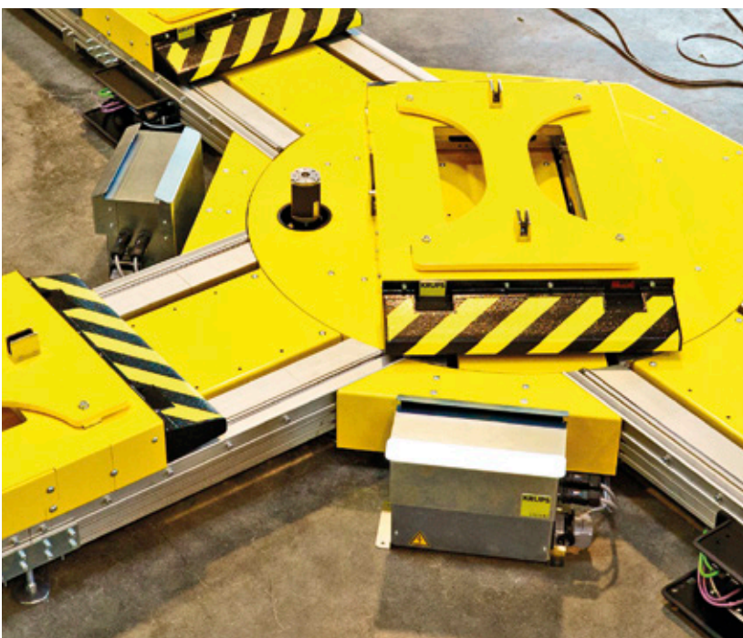
At the stoppers and other function modules the eCart system communicates with the carts via NFC
