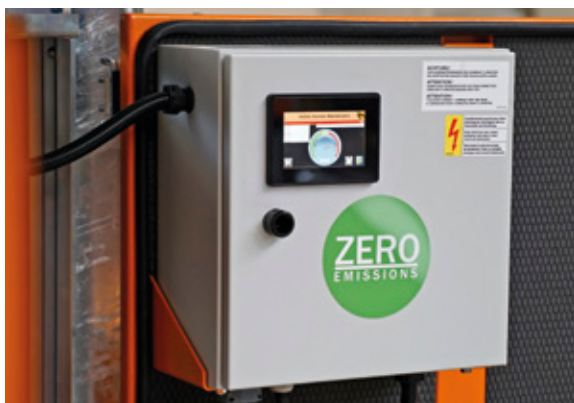
Turck's HMI/PLC TX700 combines control, visualization and edge controller for cloud connection in a single device
