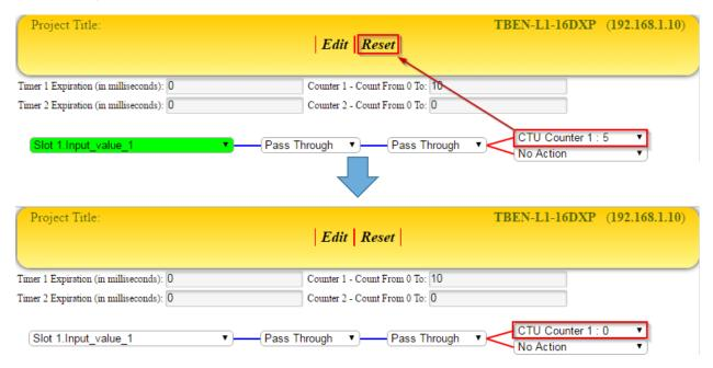
When the user clicks *Reset* while in the ARGEE PRO, the user can visually observe timers and counters resetting to zero from a more advanced screen.
