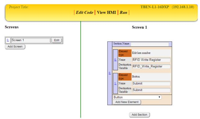
The user creates an HMI screen and adds an *Edit hex number* and *Button* element to it.
