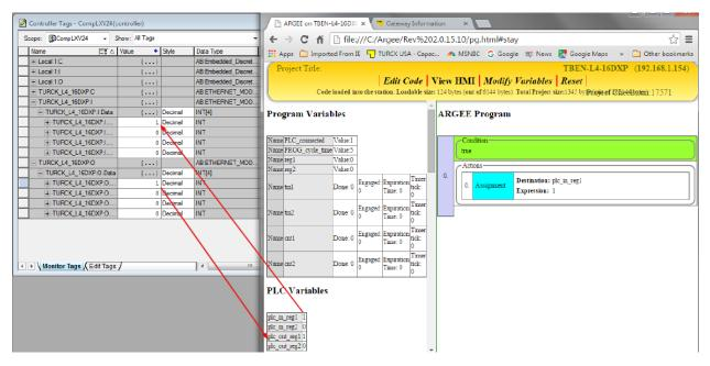
**Explaining the Example:** The user inserted the value "1" into the PLC's Output register "0", bit "0". The data transfer is verified by observing the PLC registers and the ARGEE registers.
