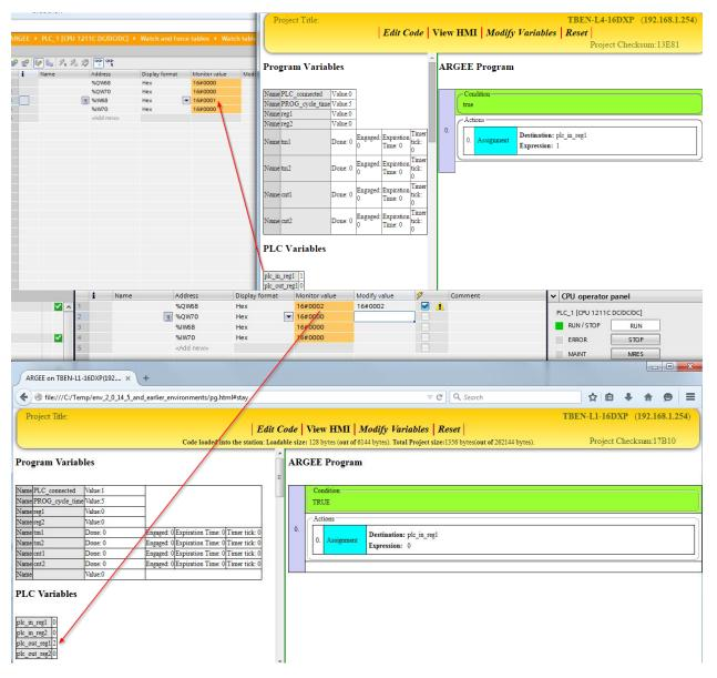
**Explaining the example:** The user inserted the value "2" into the PLC's Output register and verifies the data transfer.
