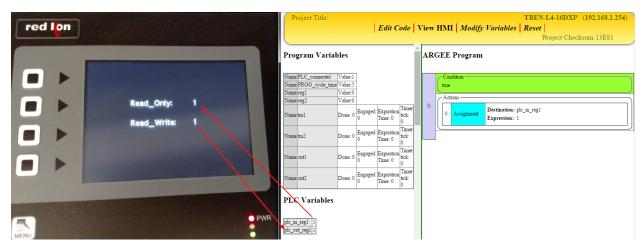
**Explaining the Example:** The user inserted the value "1" into the HMI's Output register "17409". The data transfer is verified by observing the HMI screen and the ARGEE registers.
