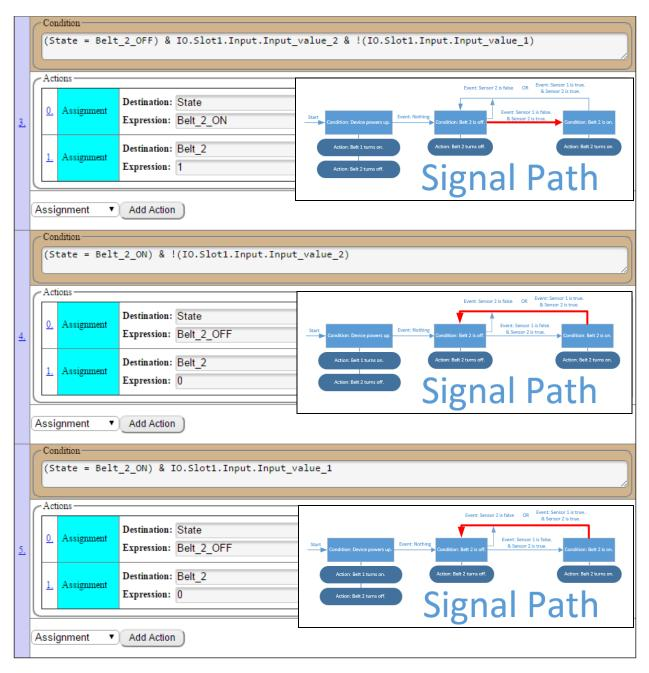
**Explaining the Example:** When the device is powered up, Belt 1 is turned on and Belt 2 is turned off. If Sensor 2 goes true (or a box shows up on Belt 2), ARGEE will check and see if Sensor 1 is true (or if a box is on Belt 1). If Sensor 1 is true then Belt 2 stays off. If Sensor 1 is false, Belt 2 turns on and clears the box on Belt 2.
