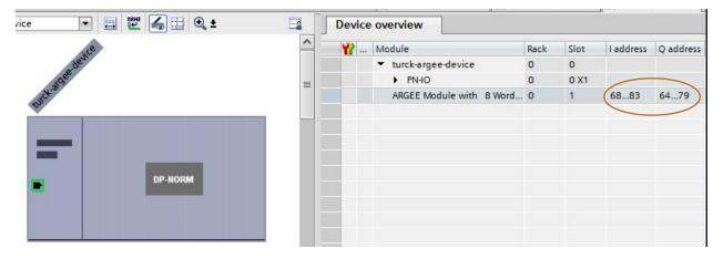
Explaining the Set up: The user defines the "I address" and "Q address" in the device overview.
