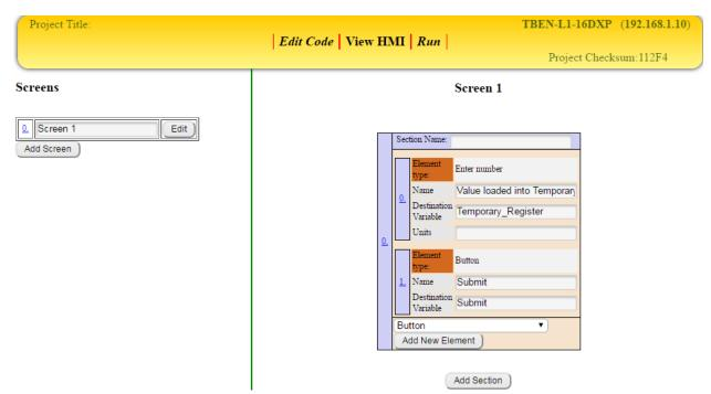
The user creates an HMI screen and adds an *Enter number* and *Button* element to it.
