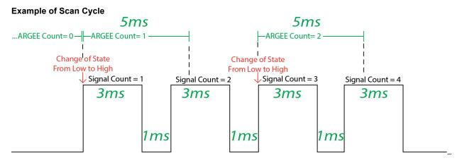
**Explaining the Example:** In this example, the user is hammering ARGEE with repeated 3 ms signals. Notice that ARGEE does not catch all the signals because the signal is occurring faster than ARGEE's Scan Cycle.
