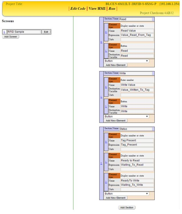
**Explaining the RFID HMI:** The user creates a "Read" section with two elements. One element displays the tag value and the other is a button that starts the "Read" operation. They also create a "Write" section with two elements. One element allows the user to enter a value and the other is a button that starts the "Write" operation. The "Status" section just displays status bits.
