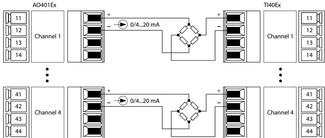
As it is supplied to the bridge, the output current of the AO401Ex output module is set to ensure that the maximum permissible compliance voltage of the AO401Ex module is not exceeded (15 VDC). Furthermore, the maximum permissible supply voltage of the bridge must not be exceeded.
