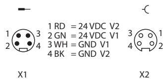
Fig. 23: TBIP-L4... – pin assignment power supply connectors
