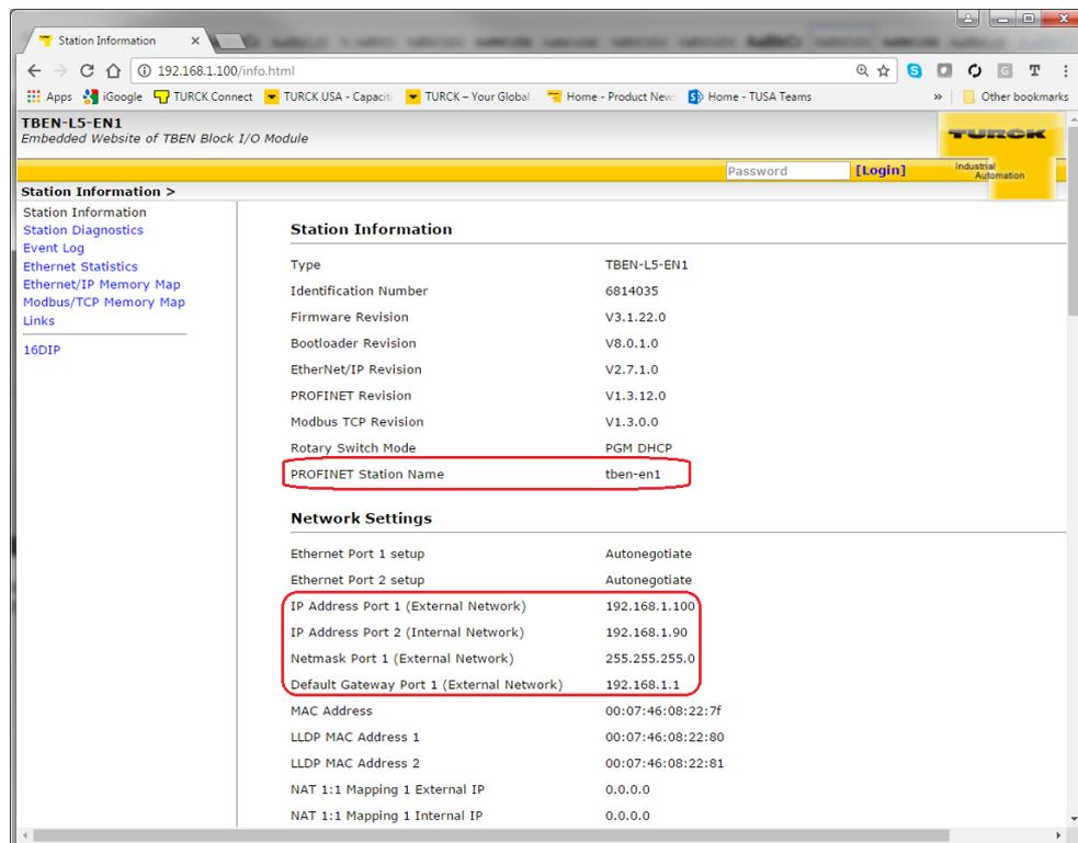
Fig. 58: Web server – setting the addresses at TBEN-L5-EN1
