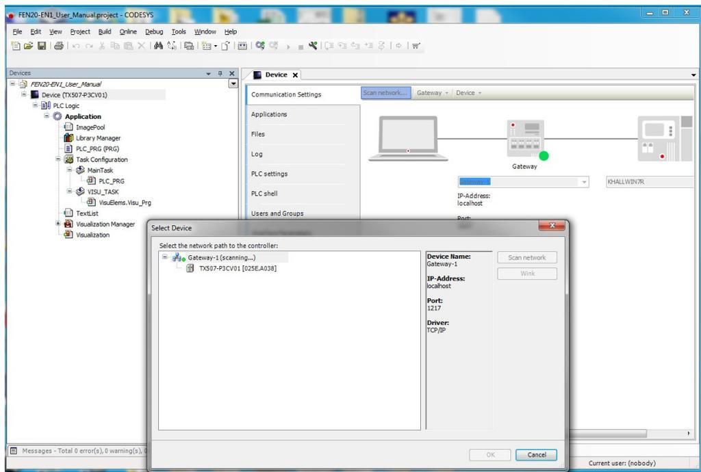
Fig. 25: CODESYS – scanning the network
