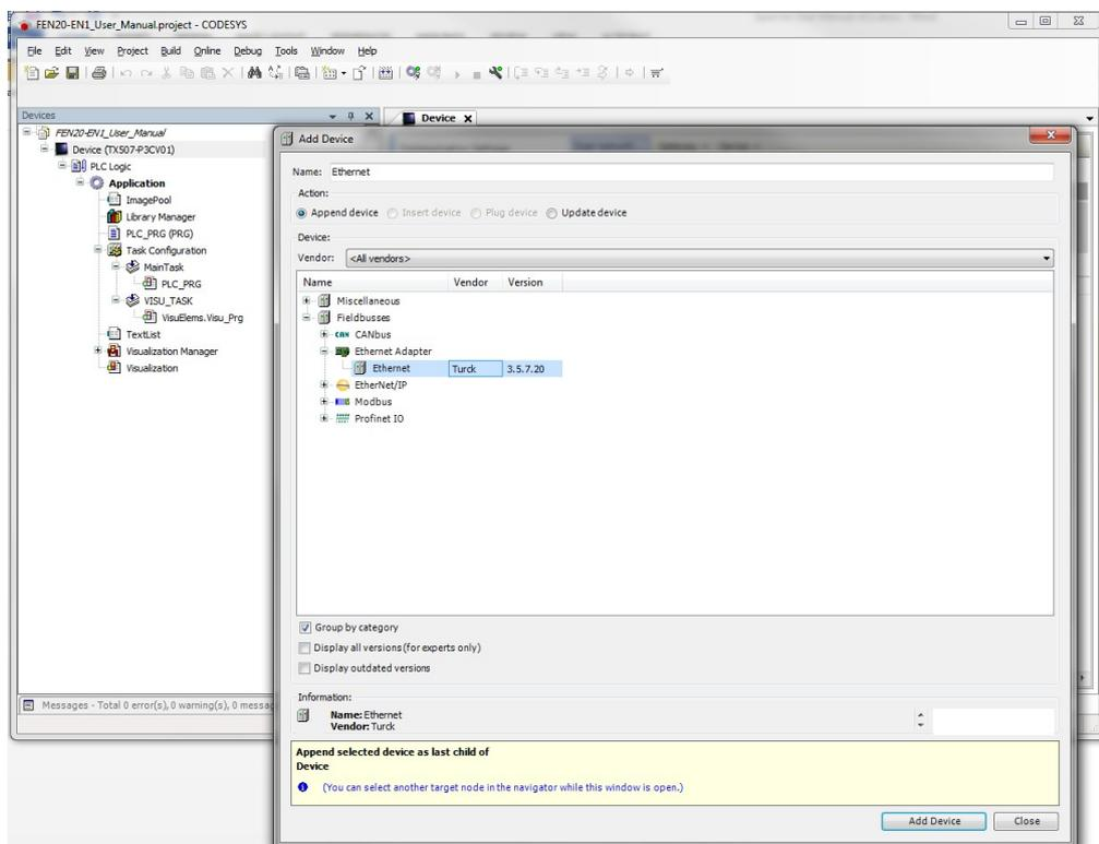
Fig. 26: CODESYS – Adding the Ethernet adapter
