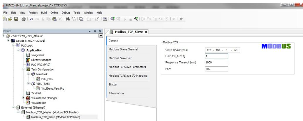
Fig. 31: CODESYS – Mapping of port 1 of FEN20-EN1 to IP address
