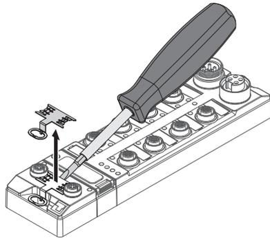
Fig. 6: Removing the grounding clamp
