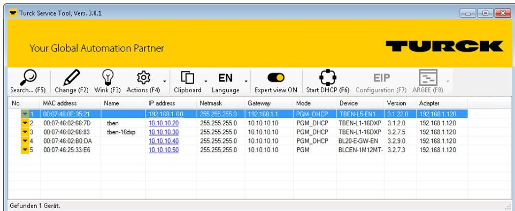
Fig. 81: Web server - Setting IP addresses
