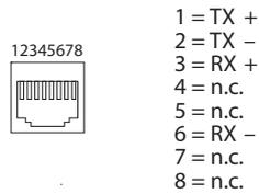
Fig. 9: Pin assignment Ethernet connectors
