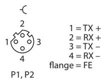
Fig. 4: Pin assignment Ethernet connectors
