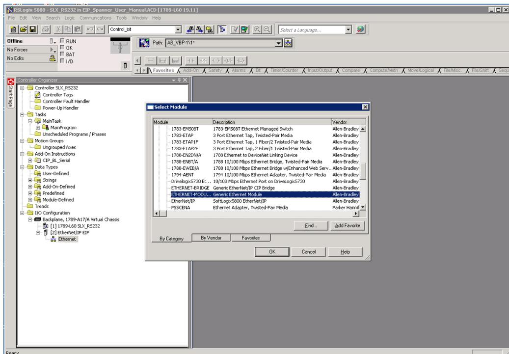
Fig. 45: RSLogix – select "Generic Ethernet Module"
