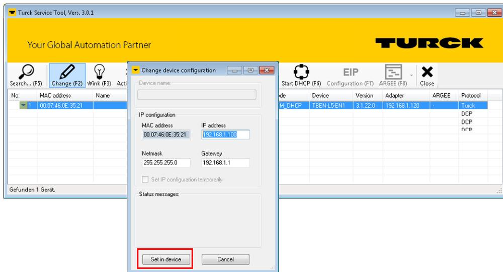
Fig. 14: Turck Service Tool – Change device configuration
