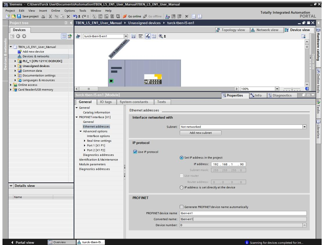
Fig. 63: TIA-Portal – assigning properties to the spanner module
