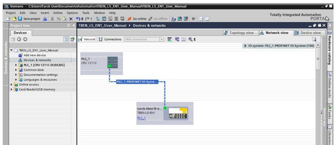
Fig. 68: TIA-Portal – connection between PLC and spanner module
