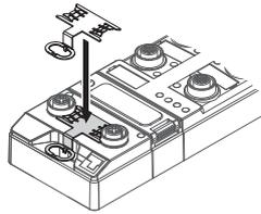
Fig. 7: Mounting the grounding clamp
