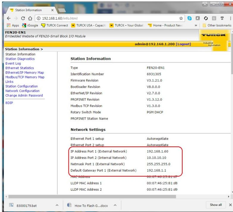
Fig. 80: Web server - Setting IP addresses
