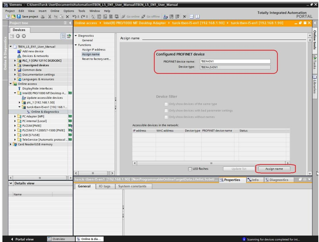
Fig. 66: TIA-Portal – assigning a PROFINET name
