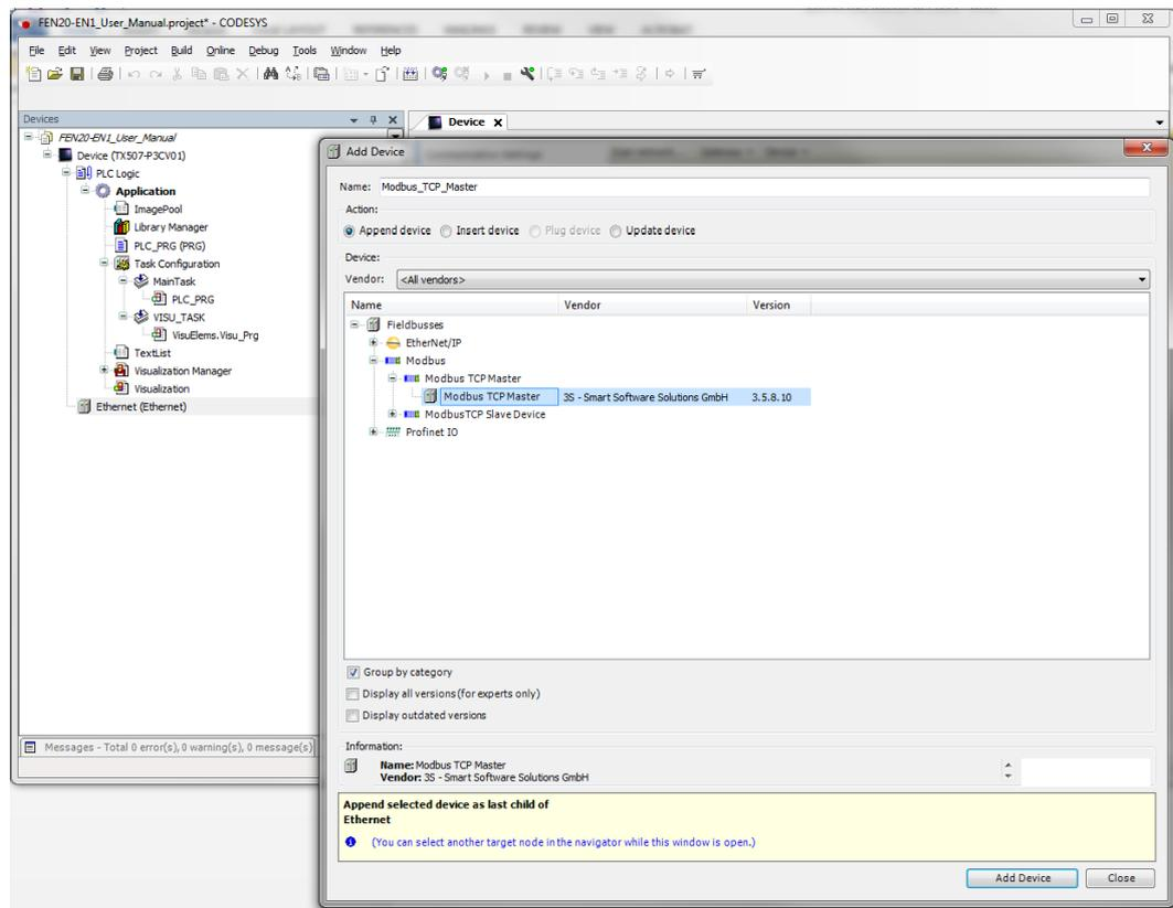
Fig. 28: CODESYS – adding the Modbus TCP Master
