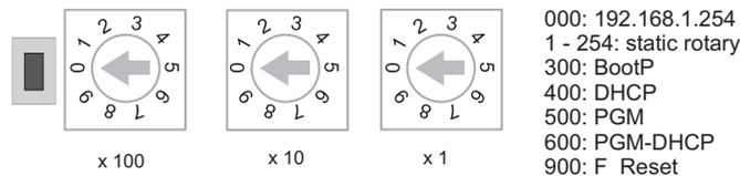
Fig. 11: Decimal rotary coding-switches for address setting
