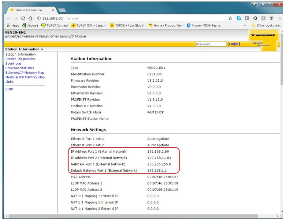
Fig. 23: Webserver – Setting the Addresses at the spanner module
