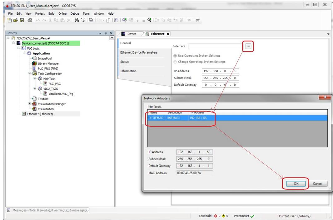
Fig. 27: CODESYS – IP address of HMI
