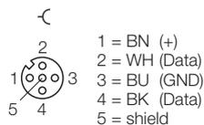
Fig. 17: .../S2501 connection cables – pin assignment of the read/write device connections
