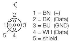
Fig. 16: .../S2500 connection cables – pin assignment of the read/write device connections
