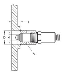
Fig. 4: Avoiding dead space and installing a leakage hole (A)
