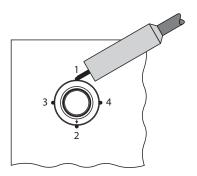
Fig. 5: Attach the welding sleeve
