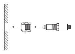
Fig. 2: Process connection with Turck process adapter
