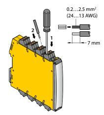
Fig. 3: Connection with spring-type terminals
