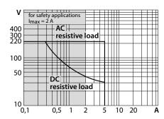
Fig. 5: Output relay load curve
