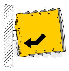
Fig. 1: Fasten the device
