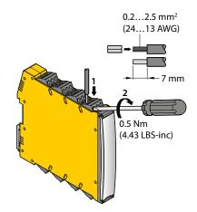
Fig. 2: Connection with screw terminals
