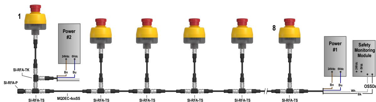
Figure 10. Option 2: Replace the terminator with a power supply. The OSSD1 and OSSD2 wires at power supply #2 must be connected to +24 V DC. If available, set the power supplies for parallel output.
