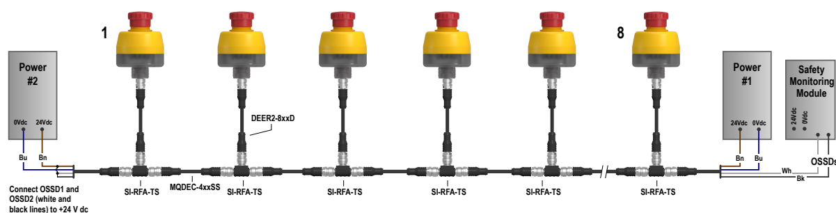
Figure 10. Option 2: Replace the terminator with a power supply. The OSSD1 and OSSD2 wires at power supply #2 must be connected to +24 V DC. If available, set the power supplies for parallel output.
