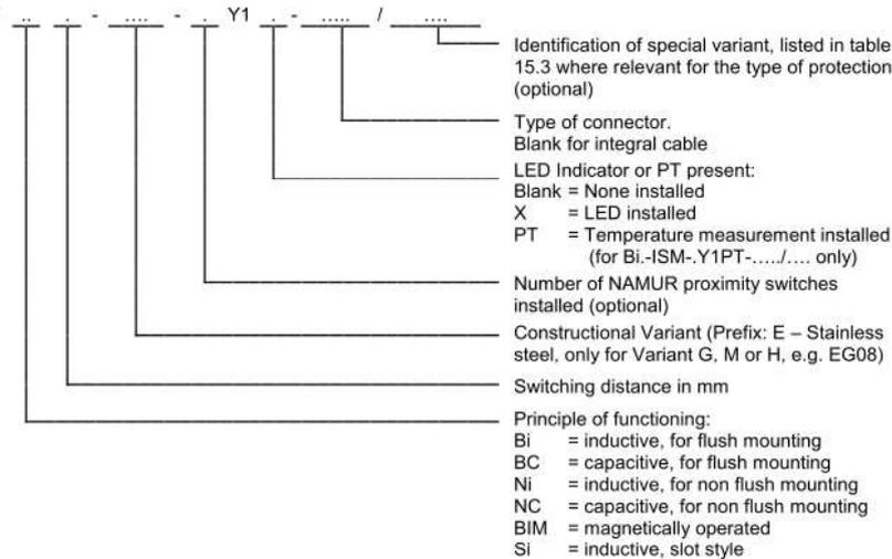
The range of two-wire proximity switches type ...-.....Y1.-...../..... consists of different designs divided into ten groups. The identification of the appropriate type group is related to the designs and can be determined from the following table:
