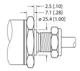
Fig. 6: Type with raised face (R10) — housing nut with thread
