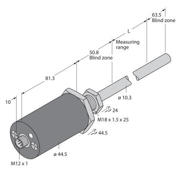
Fig. 1: LTX device dimensions with standard blind zones (in mm)
