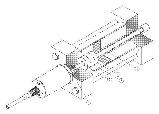
Fig. 7: Mounting the device in a hydraulic cylinder
