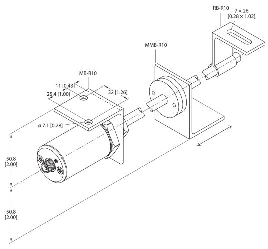
Fig. 8: Mounting a device with mounting brackets
