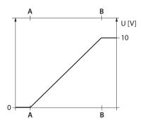
Fig. 3: Output characteristics — devices with 0...10 V voltage output
