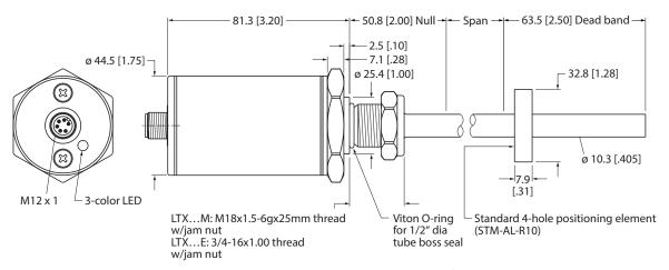
Fig. 4: Side view LTX-R10 with dimensions in mm [in] (design with raised face)
