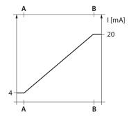
Fig. 2: Output characteristics — devices with 4...20 mA current output
