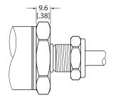
Fig. 5: Type with flat face (F10) — housing nut with thread
