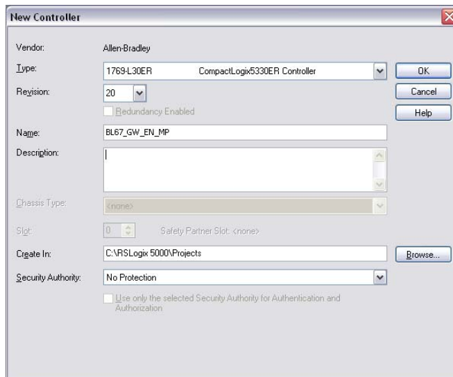
Figure 5-1: Configuration of the controller
