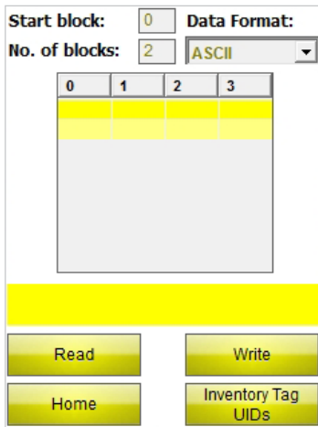
Fig. 39: Read/Write Next Tag user interface (example: 4 bytes)
