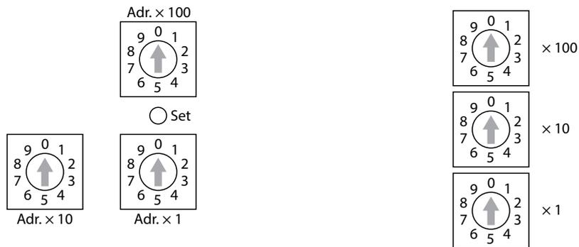
Fig. 71: Rotary coding switches on the BL20 gateway (left) and on the BL67 gateway (right)
