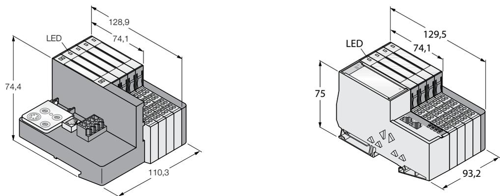
Fig. 5: BL20 interface sets (8-channel for Modbus TCP): Version with standard gateway (left) and ECO gateway (right)
