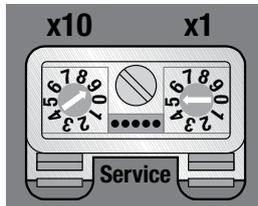
Fig. 87: Setting of the rotary coding switches for addressing in PGM mode
