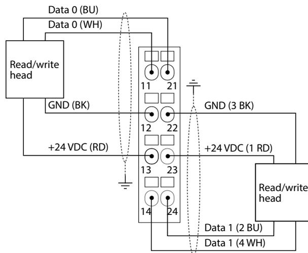
Fig. 42: Connection of HF read/write heads with .../S2503 connection cable
