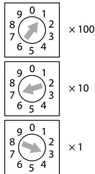
Fig. 72: Example: Setting of the rotary coding switches for the IP address 192.168.1.173 (BL67 gateway)
