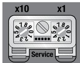
Fig. 86: Setting of the rotary coding switches for addressing in DHCP mode
