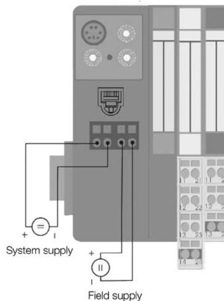
Fig. 49: BL20 gateway – Power supply terminal
