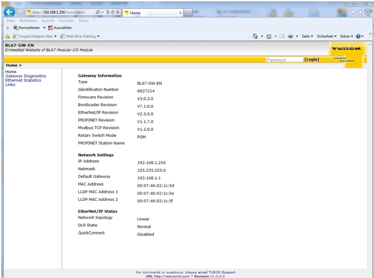
Fig. 94: Logging into the gateway – Start page (Example: BL67 gateway)
