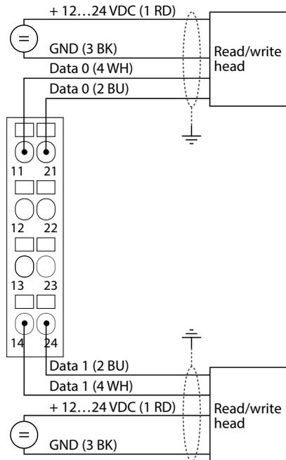
Fig. 45: Connection of UHF read/write heads with .../S2503 connection cable
