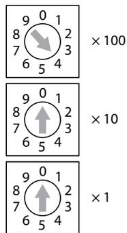
Fig. 74: Setting of the rotary coding switches for addressing in DHCP mode (BL67 gateway)
