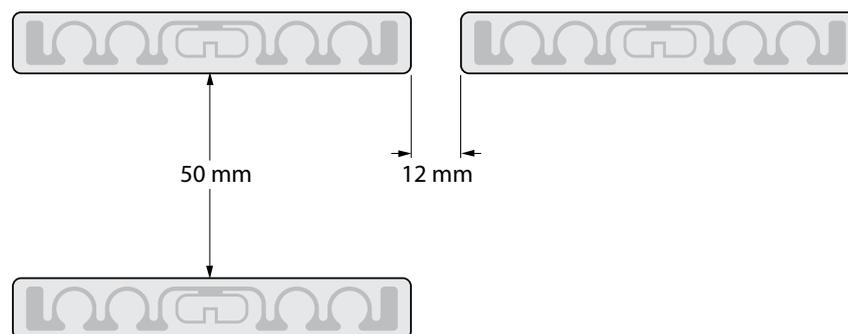
Fig. 34: Minimum distances between smart labels tags
