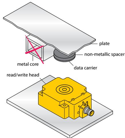
Fig. 29: Interfering metal supports
