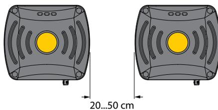
Fig. 23: Minimum distance between two read/write heads mounted next to or above each other
