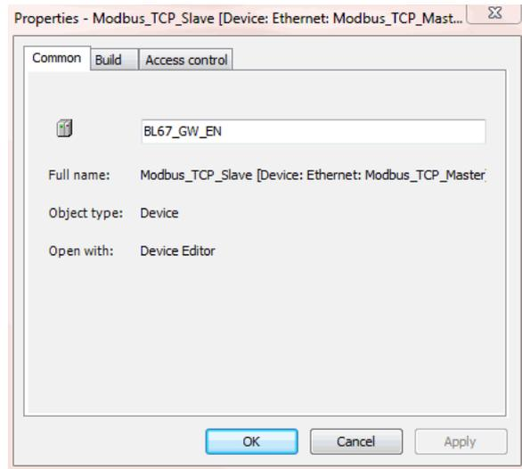
Fig. 108: Renaming Modbus TCP slaves Click the entry of the Modbus TCP slave 2 x in the project tree.
