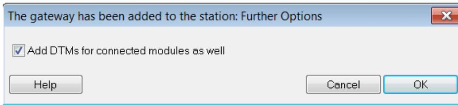
Fig. 68: Adding DTMs for the RFID electronic modules
