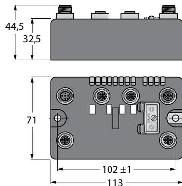
Fig. 4: Compact BL ident® interface in IP67 (BL compact) for Modbus TCP
