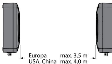
Fig. 24: Maximum distance for portal configurations
