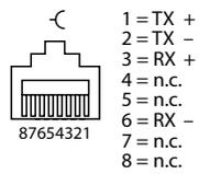
Fig. 48: BL20 gateway – Terminal layout of the RJ45 socket
