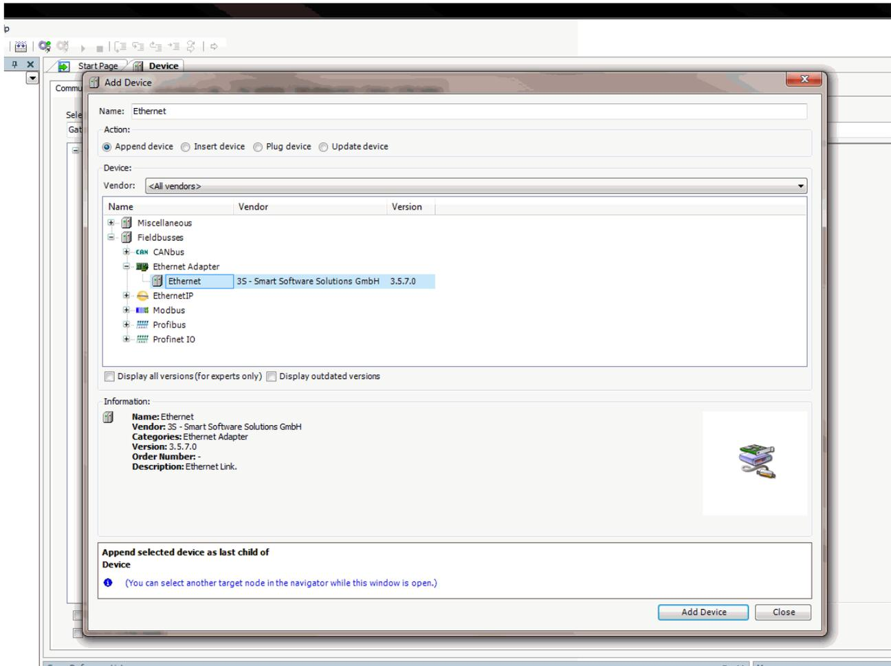
Fig. 105: Adding the Ethernet adapter as the device
