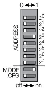
Fig. 82: Setting of the DIP switches for addressing in PGM DHCP mode (BL20 ECO gateway)
