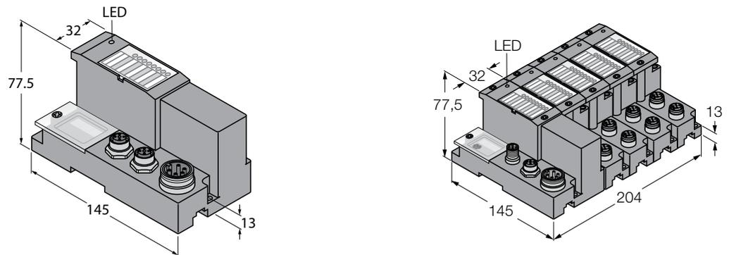
Fig. 3: BL67 gateway for Modbus TCP and BL ident® interface set with BL67 gateway and four RFID modules
