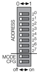
Fig. 77: DIP switches on the BL20-ECO gateway
