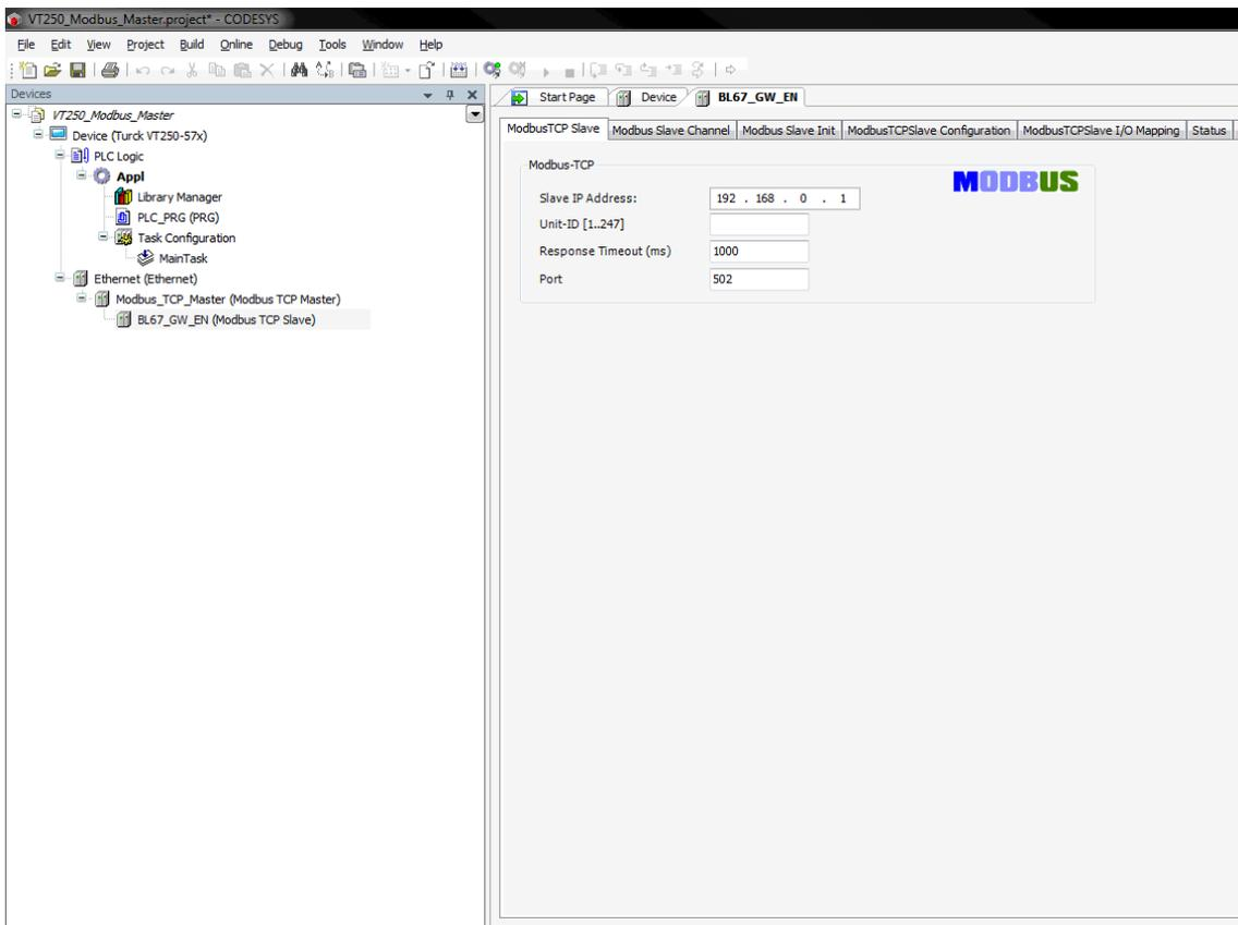
Fig. 109: Changing the IP address of the Modbus TCP slave
