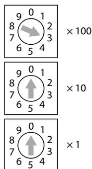
Fig. 73: Setting of the rotary coding switches for addressing in BootP mode (BL67 gateway)
