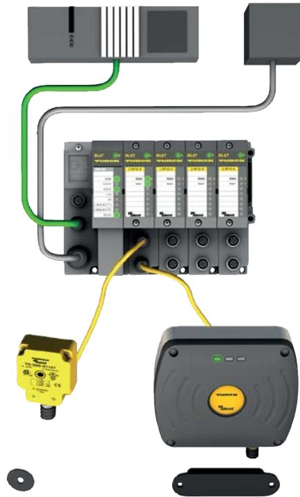
Fig. 38: Connection of BL ident® components
