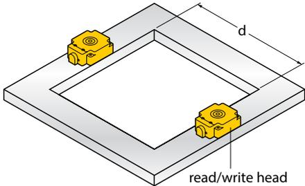
Fig. 19: Distance between two read/write heads
