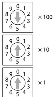
Fig. 75: Setting of the rotary coding switches for addressing in PGM mode (BL67 gateway)
