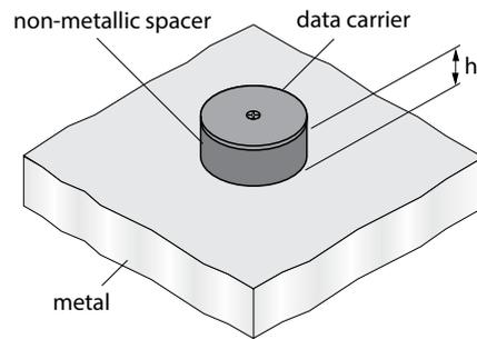
Fig. 28: Mounting with a non-metallic spacer
