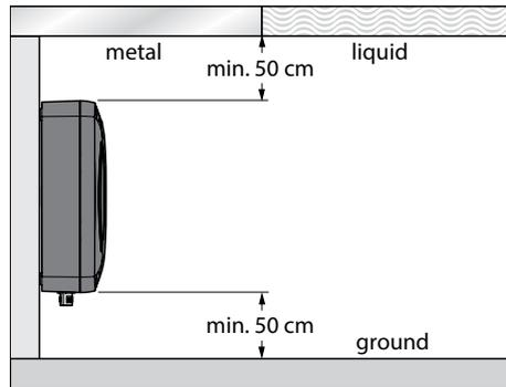
Fig. 25: Minimum distances to conductive materials for mounting read/write heads
