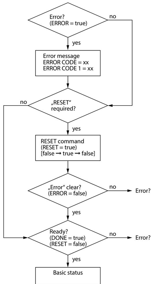
Fig. 131: Fault state flow chart
