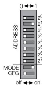
Fig. 79: Setting of the DIP switches for the IP addressing in BootP mode (BL20-ECO gateway)
