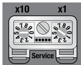
Fig. 84: Example: Setting of the rotary coding switches for the IP address 192.168.1.1
