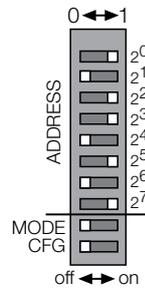
Fig. 78: Example: Setting of the DIP switches for the IP address 192.168.1.173 (BL20-ECO gateway)
