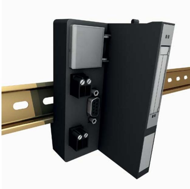
Fig. 8: Mounting BL20 gateways (example: BL20 Standard gateway)
