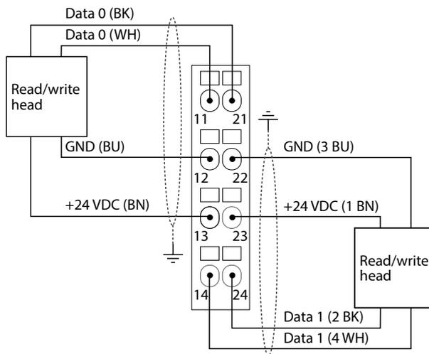
Fig. 40: Connection of HF read/write heads with .../S2500 connection cables
