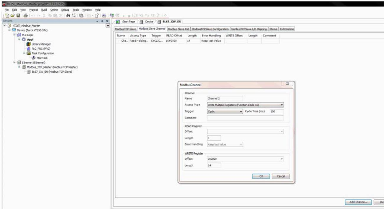
Fig. 111: Setting up a Modbus channel (WRITE register) – Example
