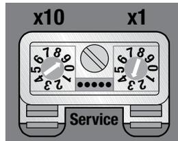
Fig. 85: Setting of the rotary coding switches for addressing in BootP mode
