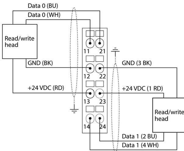
Fig. 41: Connection of HF read/write heads with .../S2501 connection cable
