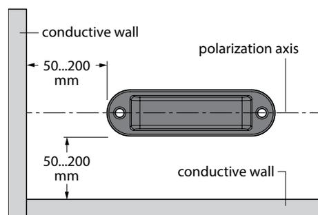
Fig. 37: Minimum distance of tags to two conductive walls
