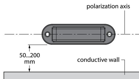
Fig. 36: Minimum distances of tags to a conductive wall, polarization axis parallel
