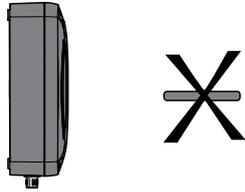
Fig. 32: Vertical alignment of tags
