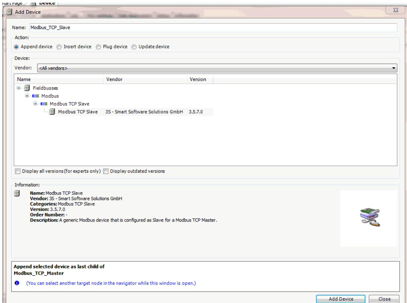
Fig. 107: Adding the Modbus TCP slaves as devices
