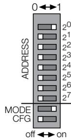
Fig. 80: Setting of the DIP switches for addressing in DHCP mode (BL20-ECO gateway)
