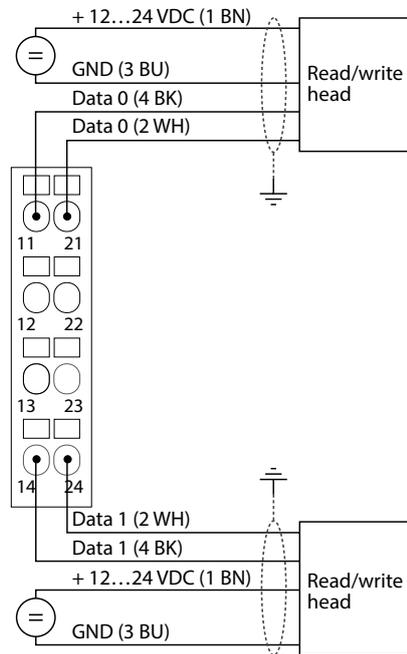
Fig. 44: Connection of UHF read/write heads with .../S2501 connection cable
