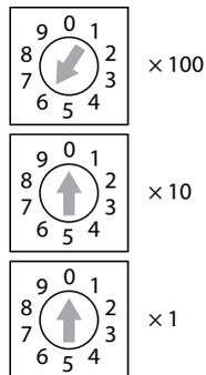
Fig. 76: Setting of the rotary coding switches for addressing in PGM-DHCP mode (BL67 gateway)
