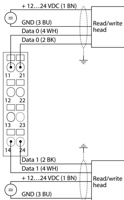
Fig. 43: Connection of UHF read/write heads with .../S2500 connection cable
