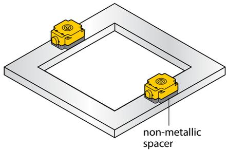
Fig. 21: Fitting a non-metallic spacer
