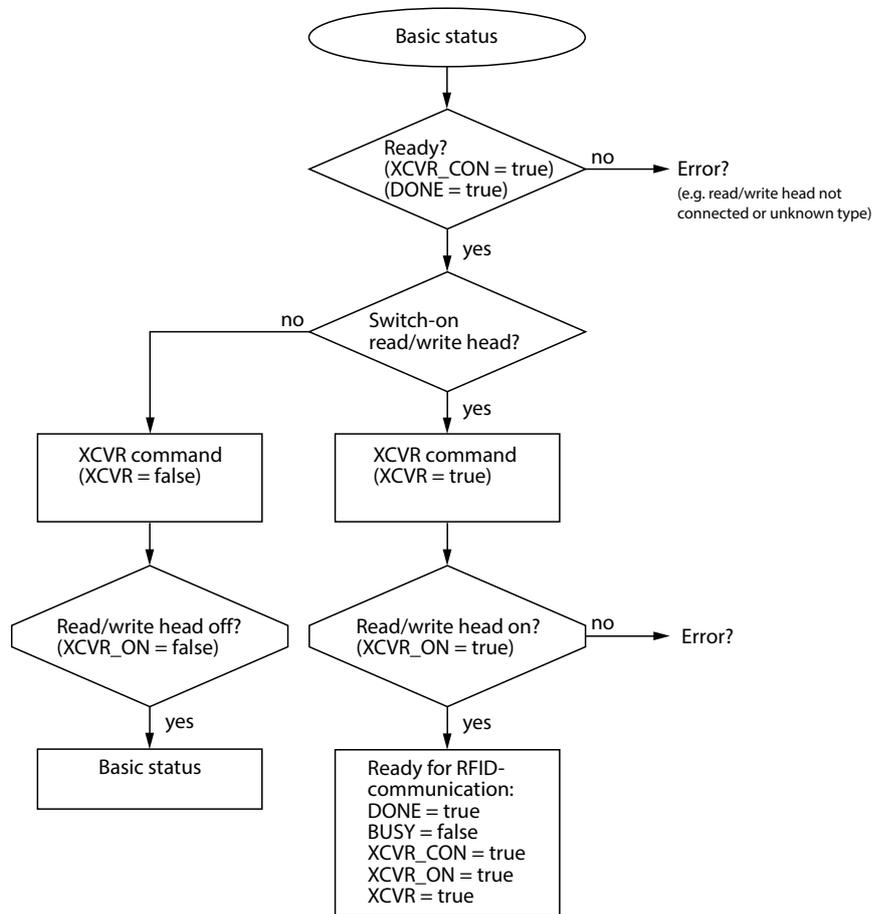
Fig. 132: Flow chart for switching the read/write head on and off
