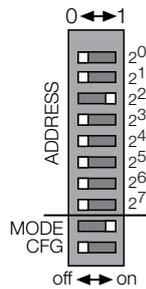
Fig. 81: Setting of the DIP switches for addressing in PGM mode (BL20 ECO gateway)
