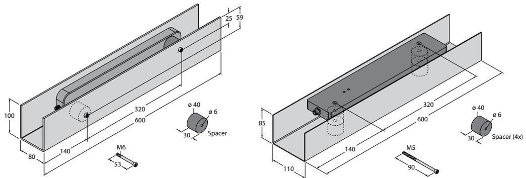
Fig. 22: Mounting the TNLr-Q80L400-... read/write head in a U profile
