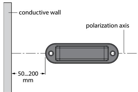
Fig. 35: Minimum distances of tags to a conductive wall, polarization axis vertical
