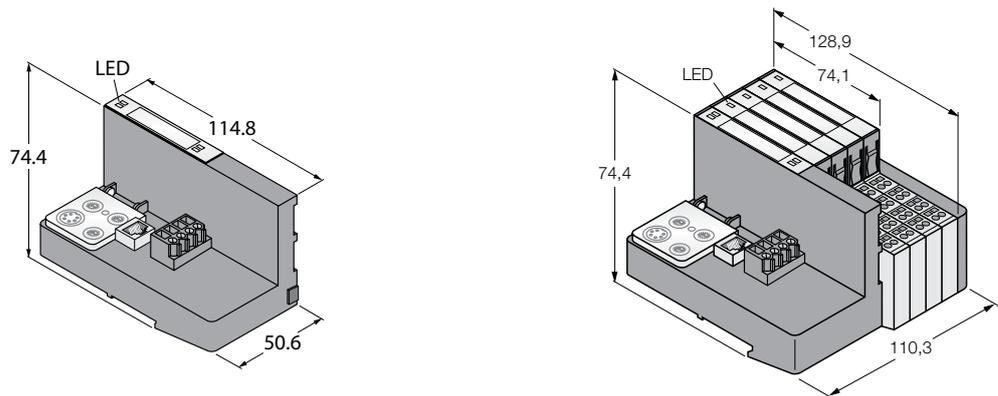
Fig. 1: BL20 standard gateway for Modbus TCP and BL ident® interface set with BL20 standard gateway and four RFID modules
