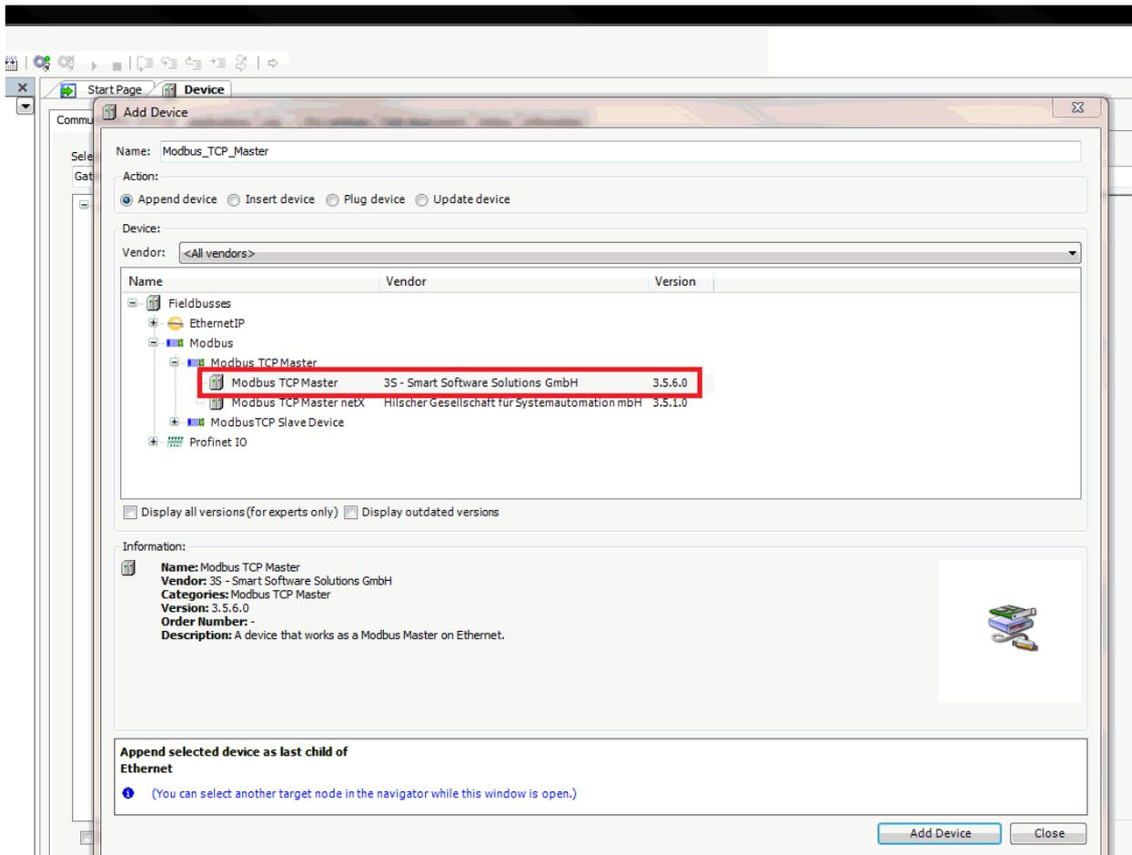
Fig. 106: Appending the Modbus master as the device
