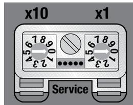
Fig. 83: Rotary coding switches on the BL compact interface
