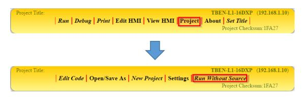
If the user clicks on *Run Without Source* and then logs out of the environment, the ARGEE program will be hidden the next time anyone logs into the block.
