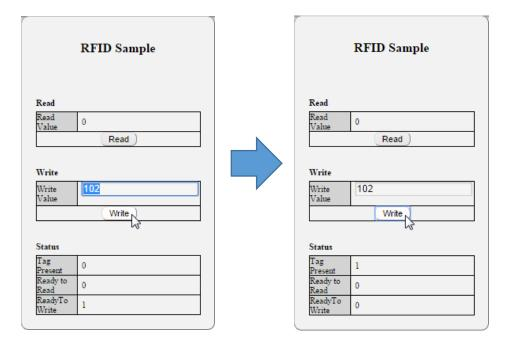
**Explaining "Write":** When the user types a value into the *Write Value* field and clicks *Write*, the "Ready To Write" status bit is true. When a tag is presented to the transceiver, the "Ready To Write" status bit goes false and the "Tag Present" bit goes true.
