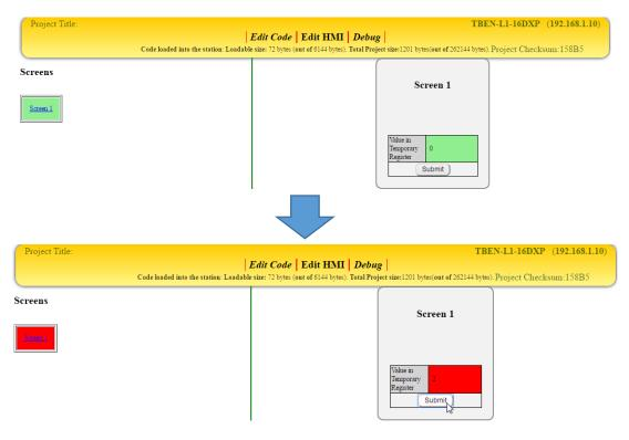
**Explaining the Example:** When the HMI first loads up, the value "0" is in Temporary\_Register. When the user presses the Submit button, the value "2" is loaded in to Temporary\_Register. The value "2" exceeds the preset maximum so the HMI goes red.
