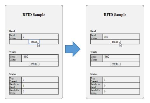
**Explaining "Read":** When the user clicks "Read", the "Ready To Read" status bit is true. When a tag is presented to the transceiver, the "Ready To Read" status bit goes false and the "Tag Present" bit goes true. The tag value is displayed in the "Read Value" field.
