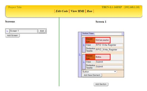
**Explaining the Example:** The user named the Edit hex number element "RFID Write Register", and then set the destination variable to be RFID\_Write\_Register. The user then named the Button element "Submit", and then set the destination variable to be Submit.
