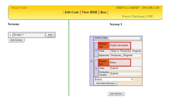
**Explaining the Example:** The user named the Display hex number "Value in Temporary Register", and then set the destination variable to be Temporary\_Register. Next, the user named the Button element "Submit" and set the destination variable to be Submit.
