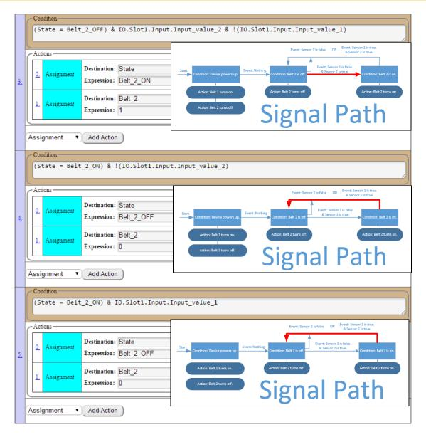
**Explaining the Example:** When the device is powered up, Belt 1 is turned on and Belt 2 is turned off. If Sensor 2 goes true (or a box shows up on Belt 2), ARGEE will check and see if Sensor 1 is true (or if a box is on Belt 1). If Sensor 1 is true then Belt 2 stays off. If Sensor 1 is false, Belt 2 turns on and clears the box on Belt 2.
