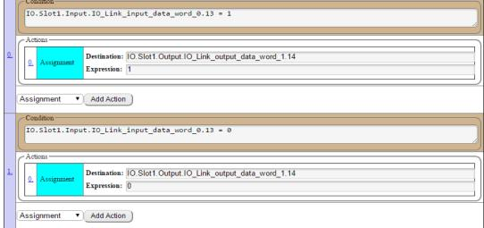
**Explaining the example:** When Connector 7 Port B on the input slave block is true, Connector 8 Port A on the output slave block is true. When Connector 7 Port B on the input slave block is false, Connector 8 Port A on the output slave block is false.
