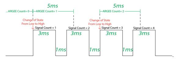
**Explaining the Example:** In this example, the user is hammering ARGEE with repeated 3 ms signals. Notice that ARGEE does not catch all the signals because the signal is occurring faster than ARGEE's Scan Cycle.
