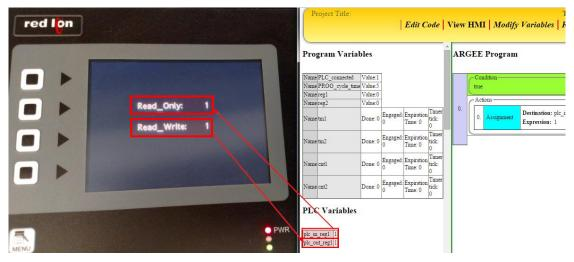
**Explaining the Example:** The user inserted the value "1" into the HMI's Output register "17409". The data transfer is verified by observing the HMI screen and the ARGEE registers.
