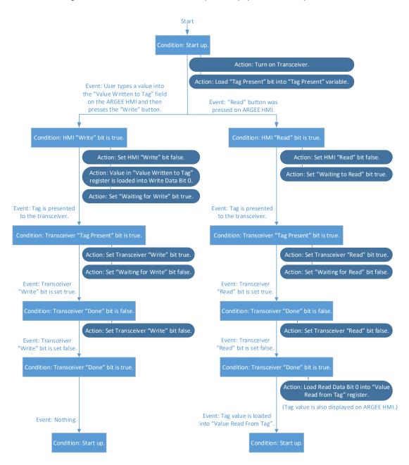
**Explaining the RFID State Machine:** When the device powers up, the transceiver gets turned on. From the ARGEE HMI screen the user can select two paths: *Read from Tag*, or *Write to Tag* path. If the user
