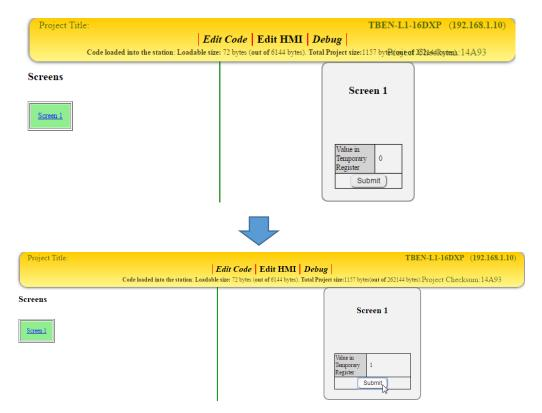
**Explaining the Example:** When the HMI first loads up, the value "0" is in Temporary\_Register. When the user presses the Submit button, the value "1" is loaded in to Temporary\_Register.
