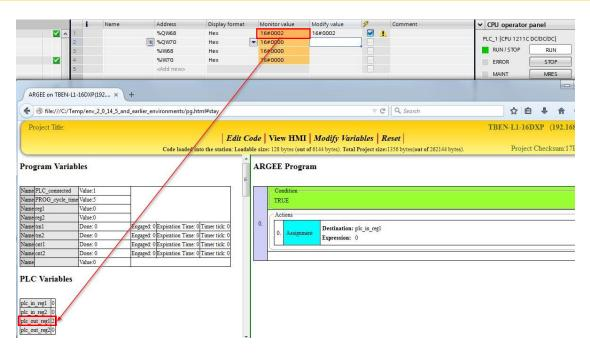
**Explaining the example:** The user inserted the value "2" into the PLC's Output register and verifies the data transfer.
