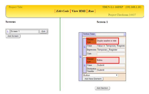
**Explaining the Example:** The user named the Display number or state element "Value in Temporary Register", and then sets the destination variable to be Temporary\_Register. Next, the user named the Button element "Submit", and then set the destination variable to be Submit.
