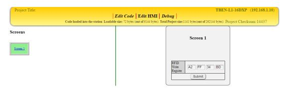
**Explaining the Example:** The user entered the hex value "A2 FF 34 BD" into the editable field. The user then clicked the Submit Button to load that value into Temporary\_Register\_1.
