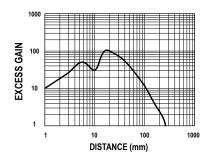
Figure 18. Excess Gain for Standard Sensitivity
