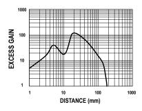
Figure 17. Excess Gain for Standard Sensitivity
