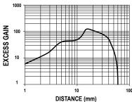
Figure 15. Excess Gain for Standard Sensitivity
