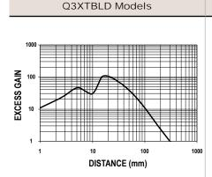
Figure 14. Excess Gain for Standard Sensitivity
