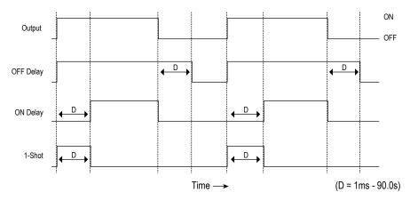
Figure 6. Output Timing Delays
