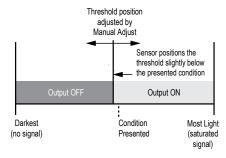
Figure 11. Light Set (Light Operate shown)
