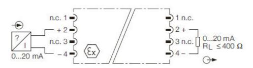
Figure 1: Block diagram - IMC-AI-\*
