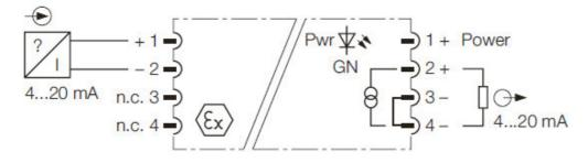
Figure 2: Block diagram – IMC-AIA-\*
