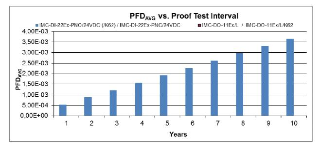
Figure 8: PFD<sub>AVG</sub> for IMC-series digital modules (diagram)
