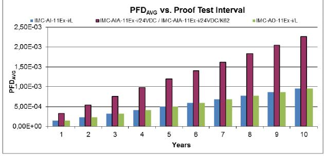
Figure 7: PFD<sub>AVG</sub> for IMC-series analogue modules (diagram)
