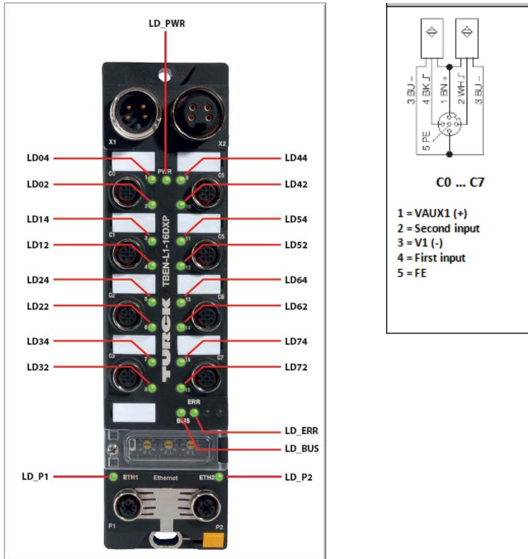
**Ethernet Ports and Device Fault LEDs**
