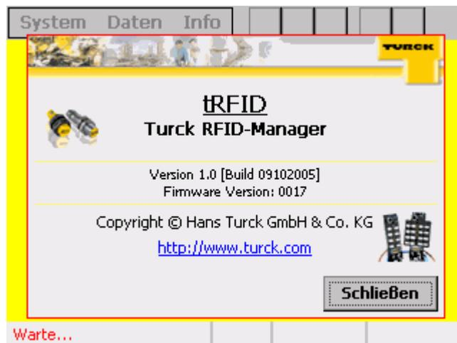
The splash screen includes important information on the software and hardware. The **Version** field shows the current version of tRFID together with the build code. The version and build code clearly identify a certain software development status. The **firmware version** indicates the version number of the loadable firmware in the RFID device.
