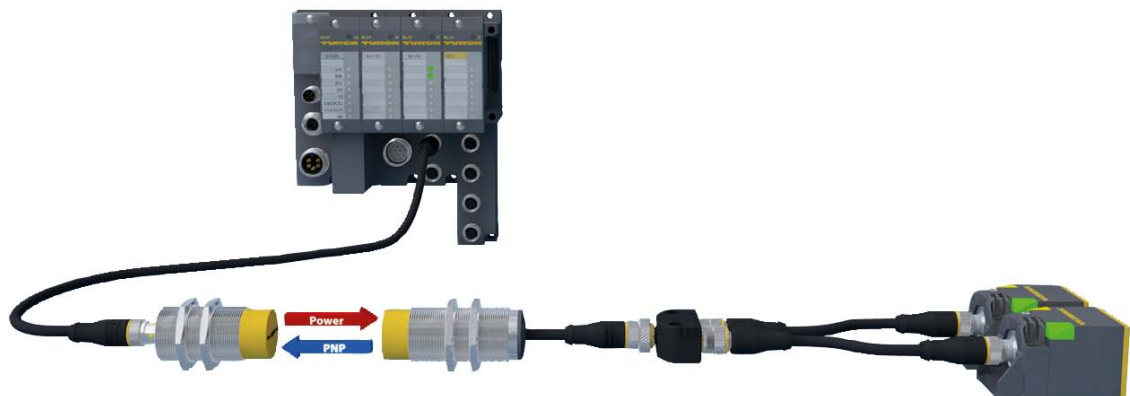
Fig. 5: Setup example for transferring 2 standard PNP signals
