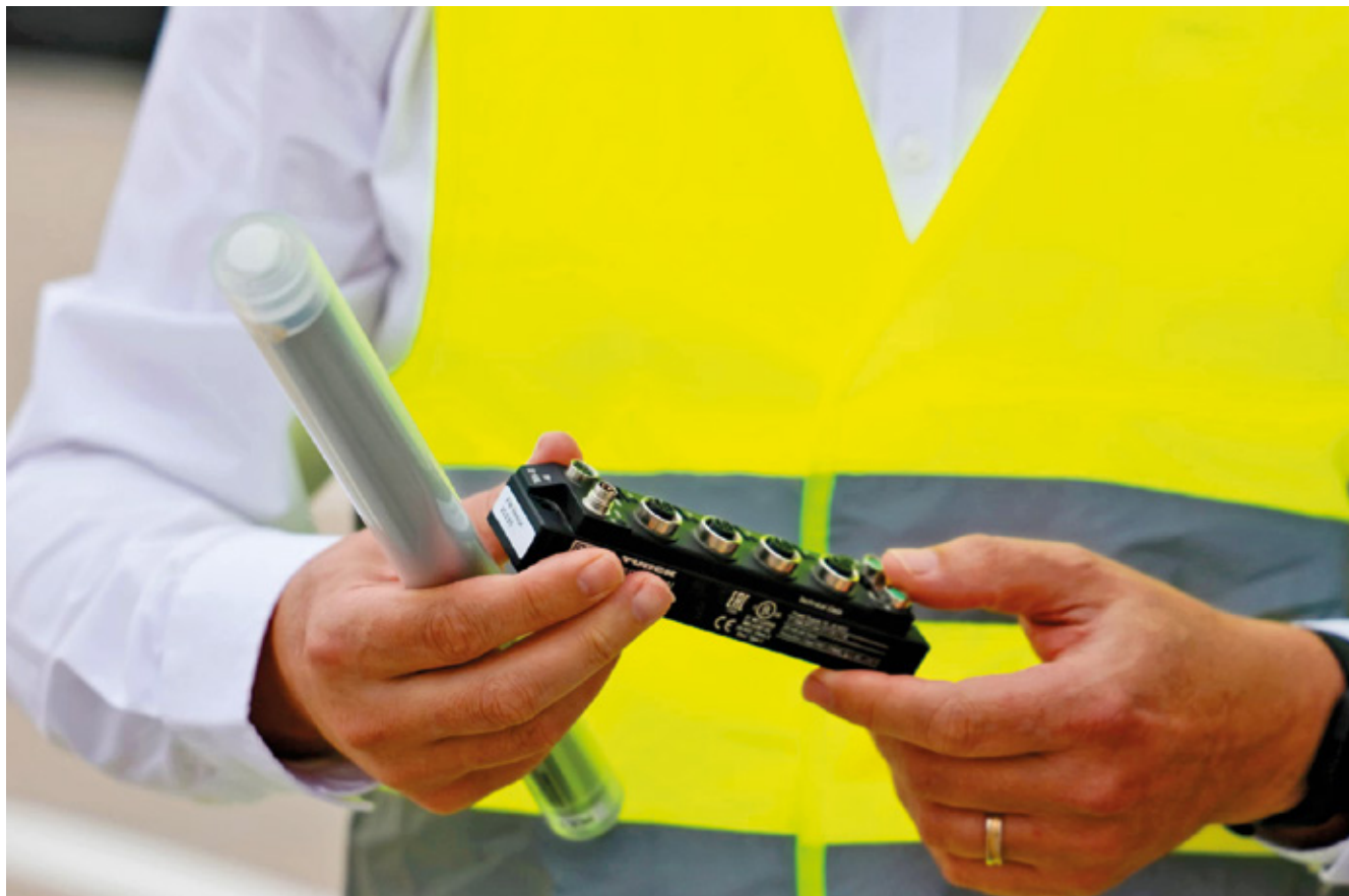
The TBEN-S2-4IOL multiprotocol I/O module is the heart of the traffic control system
