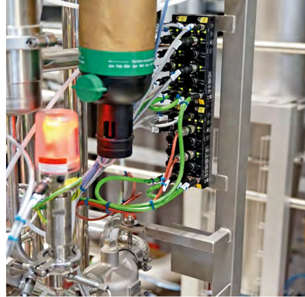
The I/O modules of the TBEN-S2 series are only 32 mm wide and allow flexible group mounting in a wide variety of locations
