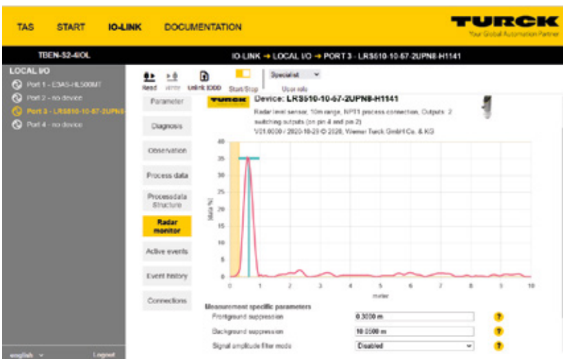
TAS Desktop: Radar Monitor simplifies sensor setup through the real-time visualization of the signal curve
