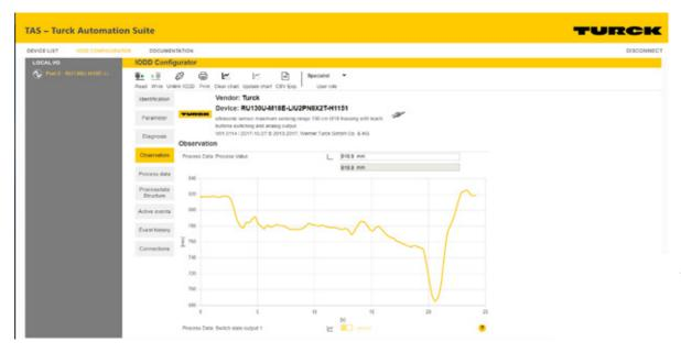
The IODD Configurator can be used, for example, to parameterize the IO-Link devices of all manufacturers
