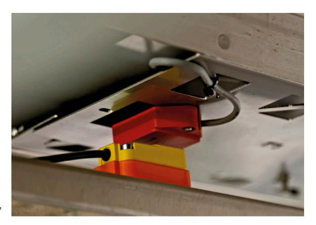
The RFID tag has a sensor connected to it which measures the temperature inside the storage container
