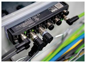
ISC CAM: The decentralized Intralox logic on Turck's robust TBEN-S block modules enables a variable conveyor layout without complex control cabinet installation
