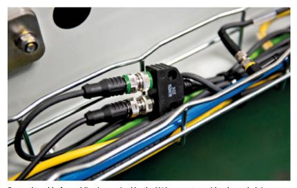
Fast and trouble-free cabling is promised by the M12 connectors with color-coded rings for poka-yoke connections
