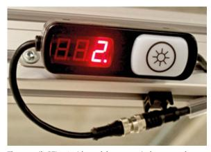
The versatile PTL110 with touch button, optical sensor and three-digit display is especially suitable for reliable operator guidance
