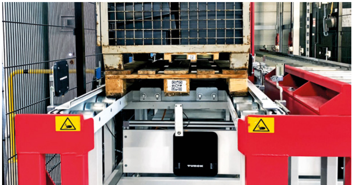
External RFID near-field antennas on the conveyor system only detect the pallet directly in front of them
