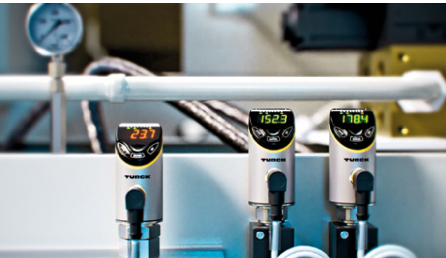
IO-Link fluid sensors monitor roller pressure and temperature for electrode calendaring
