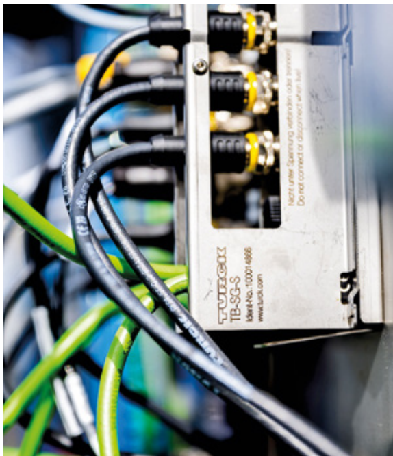
With the TB-SG stainless steel protective housings, almost all TBEN I/O modules are also approved for use in ATEX zone 2
