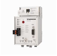
The FOC12... fiber optic media converter converts RS485 signals, e.g. from PROFIBUS-DP or Modbus RTU, on copper cables into optical signals and vice versa. The bus signals can therefore be transmitted from the safe area up to Zone 1 over long distances in a way that is intrinsically safe without potential or interference.
