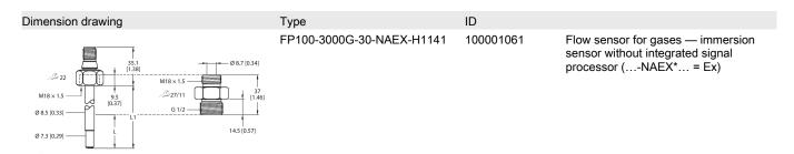
Flow sensor for gases — immersion sensor without integrated signal
