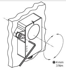
The measuring principle enables simple mounting and commissioning, for example because a metal environment does not interfere with the measuring principle. A green LED indicates whether the sensor is being supplied properly. The green flashing LED indicates that IO-Link communication is active
