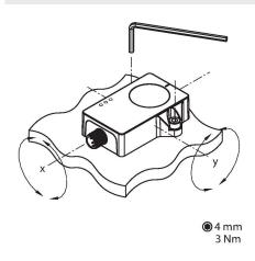
The measuring principle enables simple mounting and commissioning, for example because a metal environment does not interfere with the measuring principle. A green LED indicates whether the sensor is being supplied properly. The green flashing LED indicates that IO-Link communication is active
