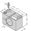
6947216 Mounting clamp for threaded barrel sensors, with dead-stop; material: PA6
