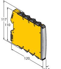
Isolating switching amplifier, 2-channel; SIL2 acc. to IEC 61508; Ex-proof version; 2 transistor outputs; input Namur signal; ON/OFF switchable monitoring of wire-break and short-circuit; toggle between NO/NC mode; signal doubling; removable screw terminals; 12.5 mm wide; 24 VDC power supply
