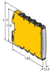
Isolating switching amplifier, 2-channel; SIL2 acc. to IEC 61508; Ex-proof version; 2 transistor outputs; input Namur signal; ON/OFF switchable monitoring of wire-break and shortcircuit; toggle between NO/NC mode; signal doubling; removable screw terminals; 12.5 mm wide; 24 VDC
