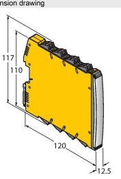
IMX12-DI01-2S-2T-0/24VDC 7580020 Isolating switching amplifier, 2-channel; SIL2 acc. to IEC 61508; Ex-proof version; 2 transistor outputs; input Namur signal; ON/OFF switchable monitoring of wire-break and short-circuit; toggle between NO/NC mode; signal doubling; removable screw terminals; 12.5 mm wide; 24 VDC
