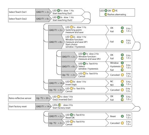
to set the window mode by teaching two limits is described below. These two limits form the switching window and can be selected freely within the detection range.
