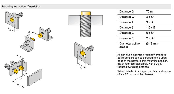
Mounting bracket for threaded barrel sensors; material: Stainless steel A2 1.4301 (AISI 304)
