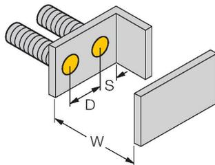
All flush mountable uprox+ threaded barrel types are also recessed mountable. Safe operation is ensured if the sensor is screwed in by half a turn.
