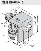
3012558 Mounting bracket, material VA 1.4401, for M10 x 1.5 thread, thread length 18 mm
