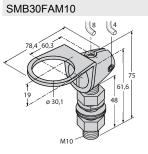
3011185 Mounting bracket, stainless steel, for M10 x 1.5 thread, thread length 30 mm
