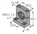
3052521 Mounting bracket, PBT black, for sensors with 30 mm thread, rotatable
