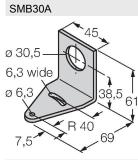
3032723 Mounting bracket, rectangular, stainless steel, for sensors with 30mm thread
