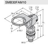
3011185 Mounting bracket, stainless steel, for M10 x 1.5 thread, thread length 30
