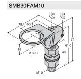
Mounting bracket, stainless steel, for M10 x 1.5 thread, thread length 30 mm
