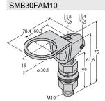
3011185 Mounting bracket, stainless steel, for M10 x 1.5 thread, thread length 30
