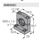
3052521 Mounting bracket, PBT black, for sensors with 30 mm thread, rotatable
