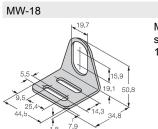
6945004 Mounting bracket for threaded barrel sensors; material: Stainless steel A2 1.4301 (AISI 304)
