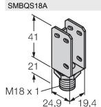
Mounting bracket, stainless steel, for 18 mm thread
