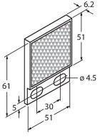
BRT-TVHG2X2 3057260 Rectangular reflective foil, reflection coefficient 0.8, ambient temperature -20 ... +60 °C, 4 sheets
