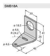
3033200 Mounting bracket, rectangular, stainless steel for sensors with 1
