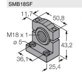
3052519 Mounting bracket, PBT black, for sensors with 18 mm thread, rotatable
