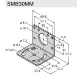
Mounting bracket, rectangular, stainless steel, for sensors with 30 mm thread, wide holes for accurate alignment
