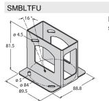
3094757 Protective housing, stainless steel, for sensors of the LTF series
