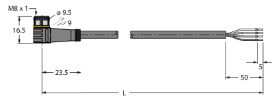
PKW4M-2/TEL 6625067 Connection cable, female M8, angled, 4-pin, cable length: 2 m, sheath material: PVC, black; cULus approval; other cable lengths and qualities available, see www.turck.com
