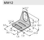
6945003 Mounting bracket for threaded barrel sensors; material: Stainless steel A2 1.4301 (AISI 304)
