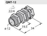
Quick-mount bracket with dead-stop; material: brass, PTFE-coated; Male thread M16  $\times$  1. Note: The switching distance of the proximity switches may change when using quick-mount brackets.
