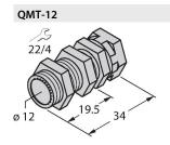
Quick-mount bracket with dead-stop; material: brass, PTFE-coated; Male thread M16  $\times$  1. Note: The switching distance of the proximity switches may change when using quick-mount brackets.
